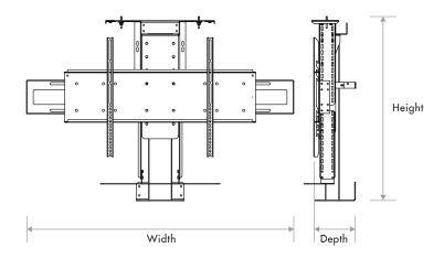
Height: 31.25" Min / 40.5" Max Adjustable in 1/4" increments Width: 37.75" Min / 54.625" Max
