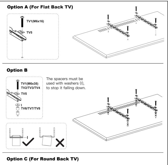
If the length of the screws is too long, the spacers can be used in multi–layer. If the installation fails after trying various methods, please contact customer service at **supportus@perlesmith.com**.
