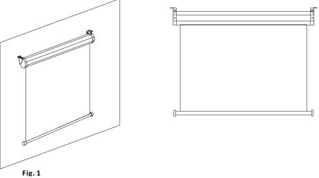
Optional installation method using the drill holes to hang the screen from the ceiling
