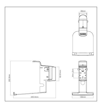
Designed to perfectly fit the Sonos Five and Play:5, this Flexson wall-mount bracket is as strong as it is discreet. The bracket securely holds the speaker in landscape position, from where it can be swivelled (up to 30 degrees left or right) and tilted (up to 20 degrees down) to angle your music to the perfect place.
