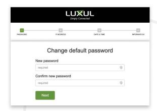
3. The default IP address method for your switch is via DHCP with a fixed failover of 192.168.0.4. Please locate your switch IP address using your Router's Connected Client list or similar function. Using the IP address that you find there, login with the default credentials.
