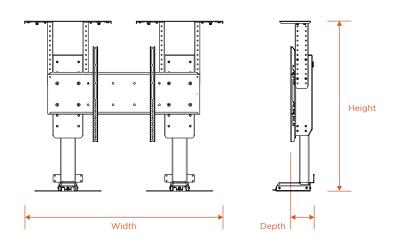
**Height:** 74.9 cm Min / 95.3 cm Max / Adjustable in 1.3 cm increments **Width:** 106.2 cm
