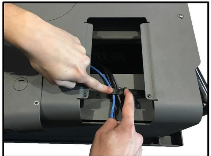
**Step 4:** Cinch the cables within the terminal using the Cable Strap. Do not completely fix the cables in place. Slack will be need to manage the cables further in a later step.
