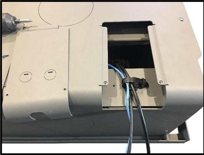
**Step 3:** Pass all AV, Integration, and Power Cables for Projector and E-500 Lift System through Cable Outlet inside the terminal.
