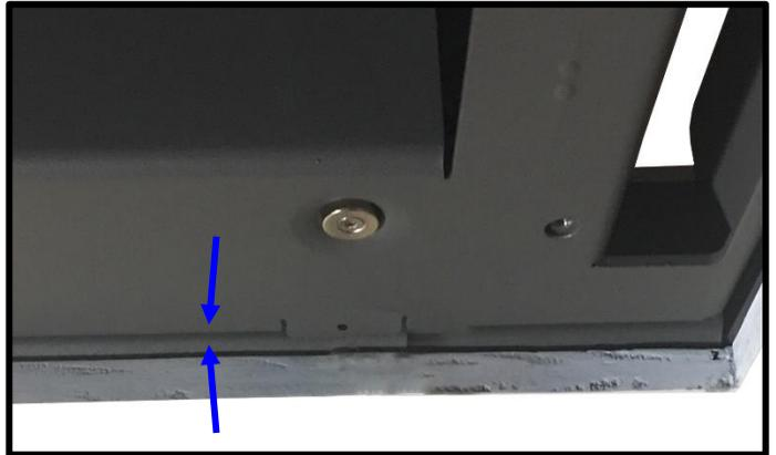
**Step 7:** Place the (4) Fine Adjustment Screws through the underside of the Actuation System into the Installation Bracket and partially fasten them using a 3mm T-Handle or Allen Key.
