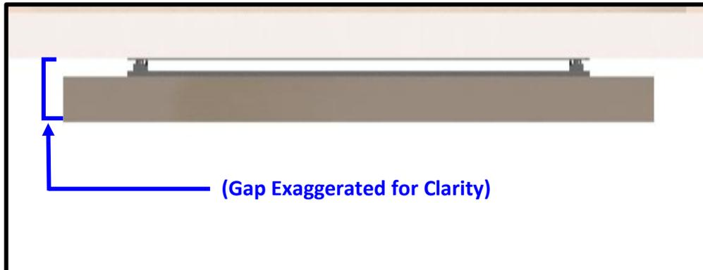
**Step 20:** Once the Ceiling Panel is flush, remove the Ceiling Panel, run the lift into the UP position, and fasten the (4) Set Screws located in the four corners of Actuation System.
