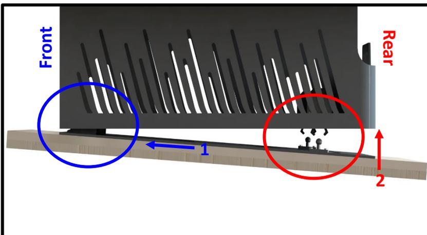
**Step 18:** Slide the Metal Tabs of the Interface Plate into the Slotted Holes on the Carrier Shroud, then press the Interface Pins into the Latches on the Carrier Shroud. Reference the arrows shown in the image to the right for direction.
