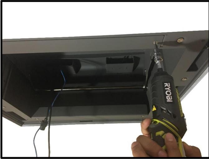
**Step 8:** Locate the Control Panel at the front of the system then, using a 3mm T-Handle or Allen Key, remove both of the Control Panel Screws to lower and expose the Wired Backup Switch.
