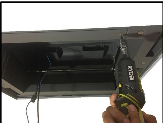
**Step 10:** Raise the Control Panel back into place then, using a 3mm T-Handle or Allen Key, fasten both of the Control Panel Screws.
