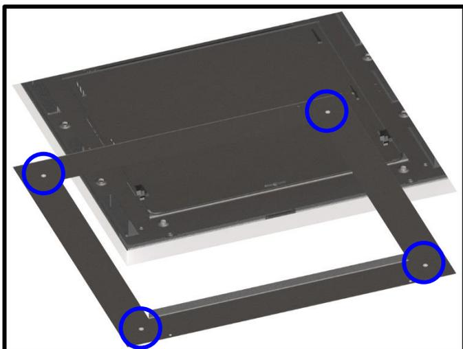
**Step 21:** With the Ceiling Panel still removed, place the Trim Ring on to the underside of the unit, and fasten it using (4) 5 x 14mm FHMS Screws.
