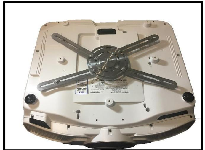
**Step 12:** Slide the Adjustment Bracket onto the Mounting Bracket then fasten the two together, using (1) 8mm Nyloc Nut and Flat Washer with a 13mm Crescent Wrench.
