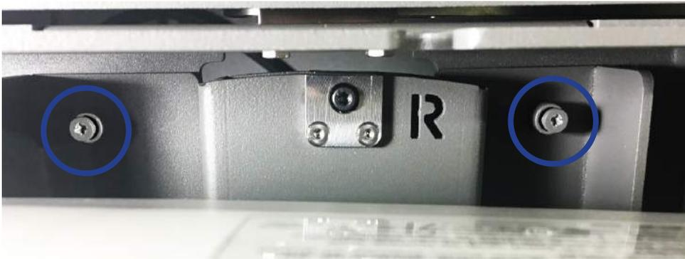
**Step 10:** Fasten the (4) Captive Hex Screws on the Projector Mount using the provided T-Handle to secure the it to the lift mechanism.
