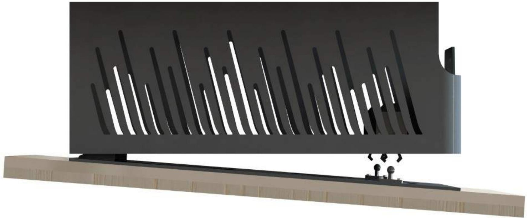
**Step 19:** Re-attach the Ceiling Panel by sliding the Metal Tabs of the Interface Plate into the Slotted Holes on the Carrier Shroud, hooking the Safety Lanyard onto the Carrier Base, then pressing the Pins into the Latches on the Carrier Shroud again.
