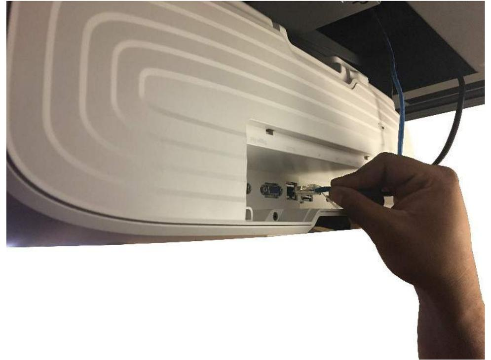
**Step 11:** Connect and manage any cables for integration or the projector and feed any excess cable back up and through the Left Cable Terminal.
