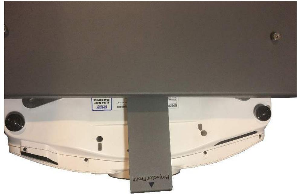
**Step 8:** Slide the Adjustment Bracket onto the Mounting Bracket stud so that the front of the Projector sits behind the flange, then fasten the two together using the previously removed M8 Nyloc Nut and Flat Washer and the provided Wrench.
