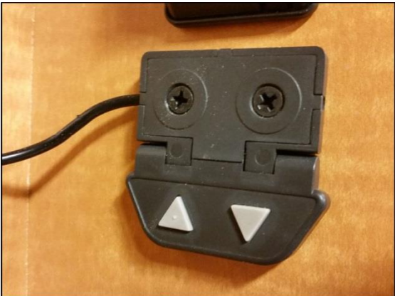
Wired Back Up Switch
