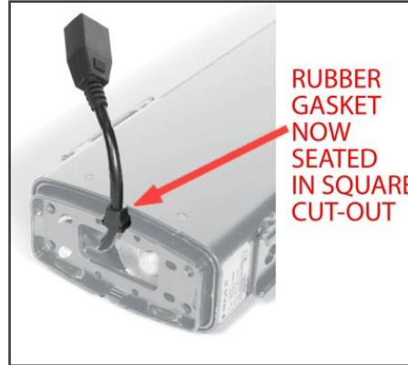
AFTER (pigtail is properly seated)
