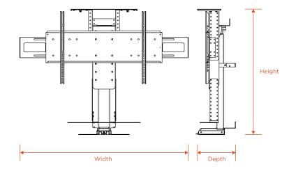
Height: 81.9 cm Min / 98.4 cm Max / Adjustable in 1.3 cm increments
