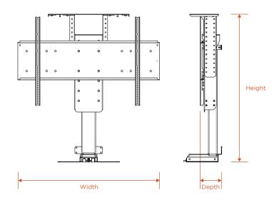
Height: 74.7 cm Min / 95 cm Max / Adjustable in 1.3 cm increments
