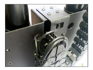
**Step 18c: Route the lower left 2.5** *Meter Motor Cable* **through the lower** *Cable Chain*. Route the *Motor Cable* through the hole on the *Column Support Bracket*. Next, slide the *Motor Cable* through the *Wire Clips* on the inside walls of the *Column Support Bracket* (previously install in step 5). Then route the *Motor Cable* through the second hole on the *Column Support Bracket*. Last, route the *Motor Cable* through the lower *Cable Chain*.
