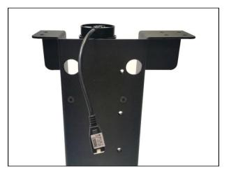
**Step 5b: Fasten the bottom of each** *Lift Column B's* **to each** *Column Support Bracket.* Flip *Lift Column B* and the *Column Support Bracket* over and align the four counter sunk holes with the four threaded holes on the bottom of *Lift Column B*. Using (8) 6mm x 20mm FHMS Screw (4 screws per *Lift Column*) attach the bottom of both *Lift Column B's* to the *Column Support Brackets*.
