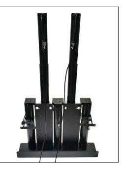
Step 10a: Attach the Screen Support (Part #4) to the upper right Lift Column. Using (4) 6mm x 16mm BHMS Screws fasten the Screen Support to the right upper Lift Column. Do not attach the left upper Lift Column, as this will be performed in Step 14b.
