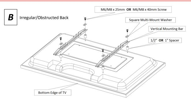
Diagram "B" installation procedure:
