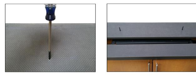
**NOTE:** You will have a ¼" tolerance (in all directions) for the placement of the Tapered Pins into your cabinet lid. There are a set of nuts on the underside of the Top Plate that allow you to adjust the position of the hole that the Taper Pins will pass through to secure the cabinet lid to the Top Plate. If you happen to position the Taper Pins a few millimeters off from your intended position, you can still make adjustments to fit properly.
