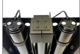
**Step 8: Temporally connect both upper** *Lift Column B's* **to the** *Control Box* (Part #8). Connect the two 4.5 meter *Motor Cables* to the pigtails of the two upper *Lift Column B's* and connect the *Control Box* and *IR or RF Controls* (depending on which controls you ordered) as shown in the wiring diagrams on pages 14 and 15. NOTE: Make sure to plug the *Motor Cables* into ports 1 and 2 on the *Control Box*.
