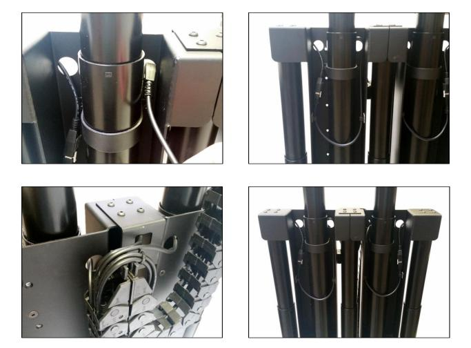
**NOTE:** Place a *Zip Tie* around the lower three *2.5 Meter Motor Cables* and a *Zip Tie* around the upper two *4.5 Meter Motor Cables*. This will aid in identifying which *Motor Cables* go to which *Lift Columns*. It is critical to not mix up the *Motor Cables* and accidently plug the upper Lift Columns into the same Control Box as the lower Lift Columns.
