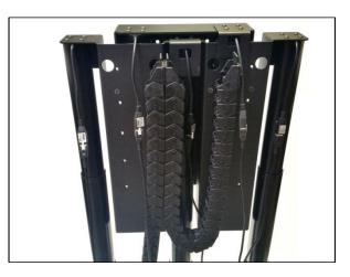
**Step 15: Route the upper two** *4.5 Meter Motor Cables* **through the upper** *Cable Chain:* Extend the upper two *Lift Columns,* as this will aid in routing the *Motor Cables*. Disconnect the two upper *Motor Cables* from the *Control Box* and route each cable down through the *Cable Chain.*
