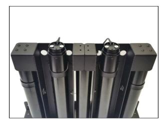
**Step 7: Attach the** *Lower Chain Bracket* (Part #16) and Upper Lift Assemblies to the top of the middle *Lift Column A*. Align the 4 holes on the *Lower Chain Bracket* and the 4 holes (2 from each Upper Lift Assembly) of the Upper Lift Assemblies with the 4 threaded holes on the top of the middle *Lift Column A* and attach using (4) 6mm x 16mm BHMS Screws. NOTE: Make sure to feed the *Lift Column A* "Pigtail" through the *Lower Chain Bracket* as seen down below.
