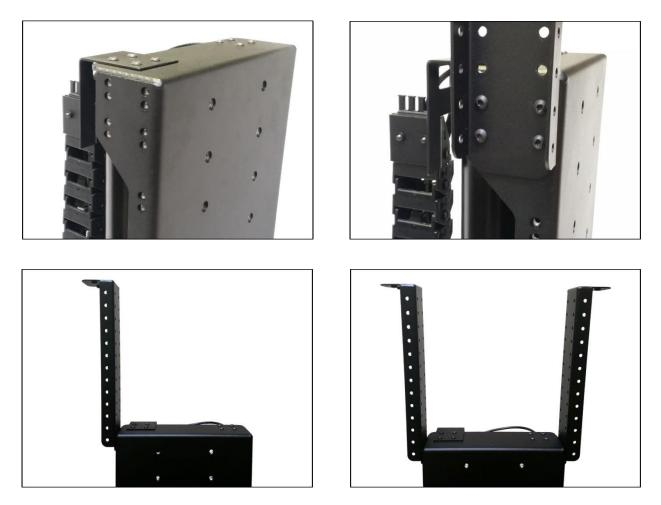
**Step 20: Attach the** *Top Plate* (Part **#5) to both** *Top Support Brackets.* Using (4) 6mm x 12mm FHMS Screws fasten the Top Plate to the top of the *Top Support Brackets*. The four countersunk holes on the *Top Plate* are offset, make sure to position the edge closes to the four countersunk holes towards the front of the lift.
