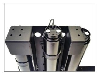
**Step 6b: Attach both Upper Lift Assemblies to the outer two** *Lift Column A's,* of the Lower Lift Assembly: Using (8) 6mm x 16mm BHMS Screws (4 screws per outer *Lift Column A's*) fasten each Upper Lift Assembly to the outer most *Lift Columns A's.* NOTE: Do not fasten the center *Lift Column A* to the Upper Lift Assemblies, as this will be completed in Step 7.
