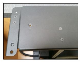
**Step 31: Mark the Tapered Pin holes on the bottom side of your lid.** With the lift in the fully retracted position, place the lid material on the *Top Plate*. Shift the lid material around until you have the lid material squared, to the top of the cabinet on all sides. Without bumping the lid or allowing the lid to shift around, raise the lift system high enough to allow you to mark the two "Nest" holes on the underside of your lid.
