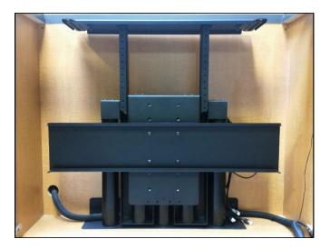
**Step 24:** Attach the *Lower Column Braces* to the cabinet. Raise the lift system until you can see the *Lower Column*
