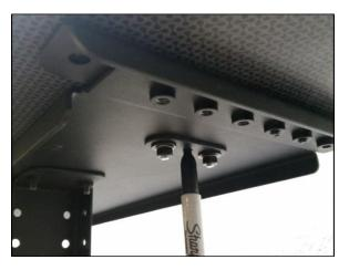
**Step 32a: Drill two ½" deep holes into the bottom side of your lid.** Using a 7/32 Drill Bit (not provided) drill two ½" holes into the bottom side of your lid in the marked positions from the previous step.
