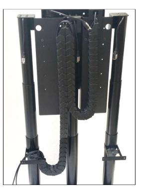
**Step 18a: Route the lower right 2.5** *Meter Motor Cable* through the lower *Cable Chain.* Route the *Motor Cable* through the hole on the *Column Support Bracket*. Next, slide the *Motor Cable* through the *Wire Clips* on the inside walls of the *Column Support Bracket* (previously install in step 5). Then route the *Motor Cable* through the second hole on the *Column Support Bracket*. Last, route the *Motor Cable* through the lower *Cable* through the *Cable* thro
