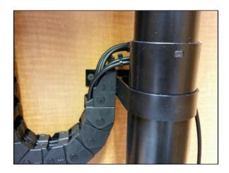
**NOTE:** Make sure to fully tighten both lower *Column Brace* rubber stops, as this will ensure there is minimal deflection from the lift system, once the TV is hung.
