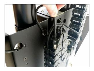
Step 18b: Route the lower center 2.5 Meter Motor Cable through the lower Cable Chain.
