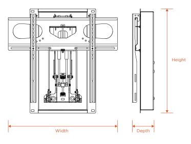
Height: 27.75" Width: 29" Depth: 5.63" (Total Mechanism) -- 2.1" (From Wall)
