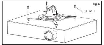
**3** Tighten the M5 x 14 screws (C) used to attach the arms to the mount base in step 1.
