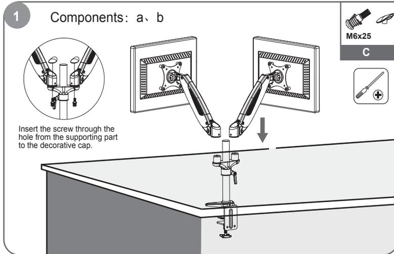
Lift the spring arm along with the monitor and put it on the supporting part.
