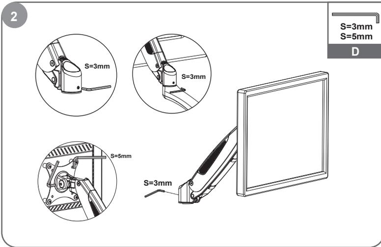
Use a hex wrench to adjust the damp for swiveling. Turn counter-clockwise to reduce damping and clockwise to increase damping.
