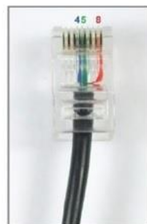
Close-up View of RJ-45 Pins
