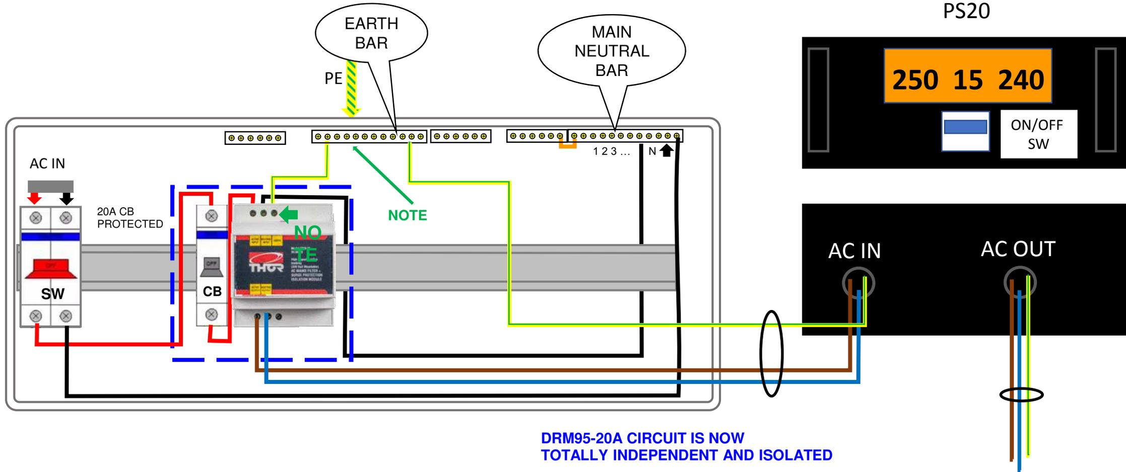
**EXAMPLE OF SWITCHBOARD USING A CB AND A DRM 95-20A CONNECTED TO A PS20**
