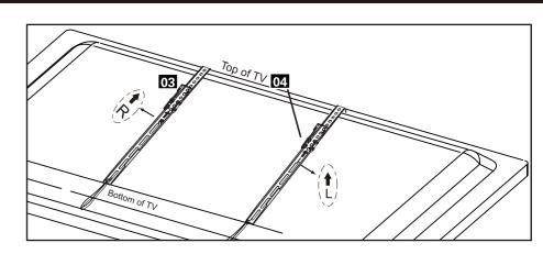
Adjust the tilting angle with the Screw driver for both 04 and 03.
