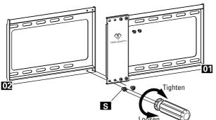
Remove the connection screws **s** x4, and Assemble the wall plate sections 01 and 02 with the removed connection plate
